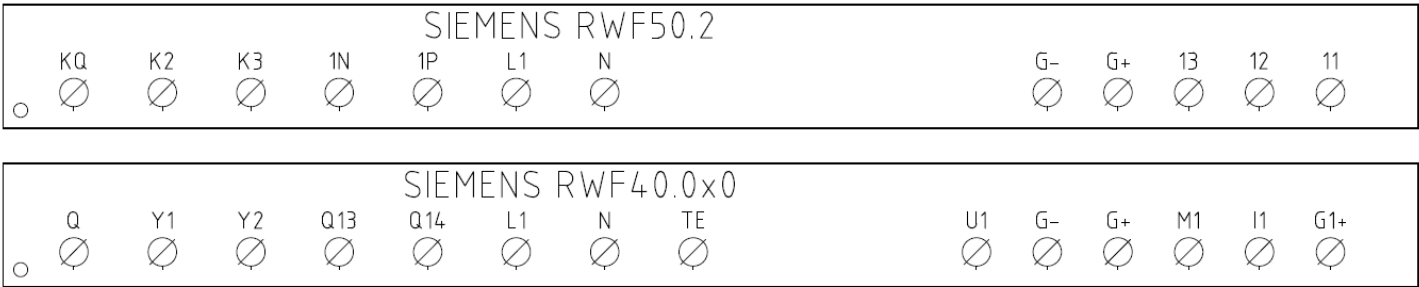
Matches terminals between RWF50.2 and RWF40.0x0
